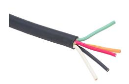
Southwire portable cord, unshielded, SOOW, 600V, 5 conductors (includes ground), 16 AWG, EPDM thermoset rubber conductor insulation material, black, white, red, green and orange, CPE thermoset rubber jacket, black, cut to length.
