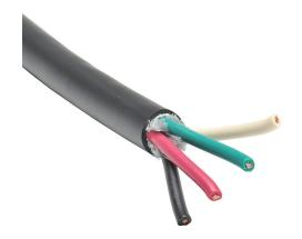
Southwire portable cord, unshielded, SOOW, 600V, 4 conductors (includes ground), 16 AWG, EPDM thermoset rubber conductor insulation material, black, white, red and green, CPE thermoset rubber jacket, black, cut to length.
