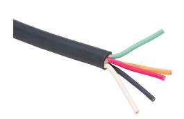
Southwire portable cord, unshielded, SOOW, 600V, 5 conductors (includes ground), 14 AWG, EPDM thermoset rubber conductor insulation material, black, white, red, green and orange, CPE thermoset rubber jacket, black, cut to length.
