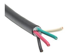
Southwire portable cord, unshielded, SOOW, 600V, 4 conductors (includes ground), 14 AWG, EPDM thermoset rubber conductor insulation material, black, white, red and green, CPE thermoset rubber jacket, black, cut to length.
