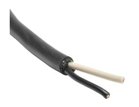
Southwire portable cord, unshielded, SOOW, 600V, 2 conductors, 14 AWG, EPDM thermoset rubber conductor insulation material, black and white, CPE thermoset rubber jacket, black, cut to length.
