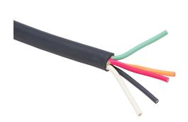
Southwire portable cord, unshielded, SOOW, 600V, 5 conductors (includes ground), 12 AWG, EPDM thermoset rubber conductor insulation material, black, white, red, green and orange, CPE thermoset rubber jacket, black, cut to length.
