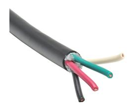
Southwire portable cord, unshielded, SOOW, 600V, 4 conductors (includes ground), 12 AWG, EPDM thermoset rubber conductor insulation material, black, white, red and green, CPE thermoset rubber jacket, black, cut to length.
