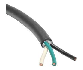
Southwire portable cord, unshielded, SOOW, 600V, 3 conductors (includes ground), 12 AWG, EPDM thermoset rubber conductor insulation material, black, white and green, CPE thermoset rubber jacket, black, cut to length.
