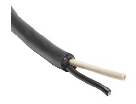
Southwire portable cord, unshielded, SOOW, 600V, 2 conductors, 12 AWG, EPDM thermoset rubber conductor insulation material, black and white, CPE thermoset rubber jacket, black, cut to length.
