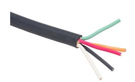
Southwire portable cord, unshielded, SOOW, 600V, 5 conductors (includes ground), 10 AWG, EPDM thermoset rubber conductor insulation material, black, white, red, green and orange, CPE thermoset rubber jacket, black, cut to length.
