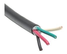
Southwire portable cord, unshielded, SOOW, 600V, 4 conductors (includes ground), 10 AWG, EPDM thermoset rubber conductor insulation material, black, white, red and green, CPE thermoset rubber jacket, black, cut to length.
