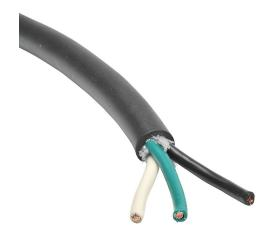
Southwire portable cord, unshielded, SOOW, 600V, 3 conductors (includes ground), 10 AWG, EPDM thermoset rubber conductor insulation material, black, white and green, CPE thermoset rubber jacket, black, cut to length.
