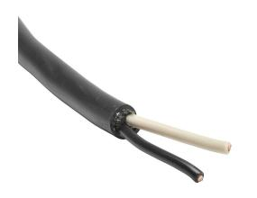
Southwire portable cord, unshielded, SOOW, 600V, 2 conductors, 10 AWG, EPDM thermoset rubber conductor insulation material, black and white, CPE thermoset rubber jacket, black, cut to length.
