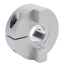
Sung-II Machinery drive coupling hub, Oldham, aluminum alloy, clamp, size 70, 1in bore. Requires SOH-70-DISC torque disc.
