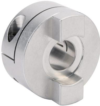
Sung-II Machinery drive coupling hub, Oldham, aluminum alloy, clamp, size 57, 19mm bore. Requires SOH-57-DISC torque disc.
