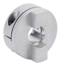
Sung-II Machinery drive coupling hub, Oldham, aluminum alloy, clamp, size 43, 5/8in bore. Requires SOH-43-DISC torque disc.
