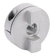
Sung-II Machinery drive coupling hub, Oldham, aluminum alloy, clamp, size 43, 12mm bore. Requires SOH-43-DISC torque disc.
