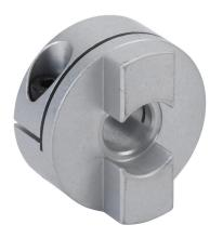
Sung-II Machinery drive coupling hub, Oldham, aluminum alloy, clamp, size 25, 8mm bore. Requires SOH-25-DISC torque disc.
