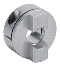
Sung-II Machinery drive coupling hub, Oldham, aluminum alloy, clamp, size 20, 5/16in bore. Requires SOH-20-DISC torque disc.
