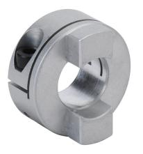
Sung-II Machinery drive coupling hub, Oldham, aluminum alloy, clamp, size 20, 10mm bore. Requires SOH-20-DISC torque disc.
