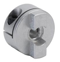
Sung-II Machinery drive coupling hub, Oldham, aluminum alloy, clamp, size 16, 4mm bore. Requires SOH-16-DISC torque disc.
