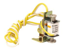
Eaton field installable shunt trip, 110-240 VAC/110-125 VDC coil voltage, 18in pigtail. For use with AutomationDirect (Eaton) 400A frame MCCBs.
