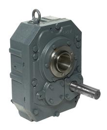
IronHorse heavy-duty shaft mounted gearbox, 25:1 ratio, 1-7/16in shaft input, tapered bore, maximum motor 20hp, 2-7/16in maximum output shaft diameter, size 4 frame, cast iron housing.
