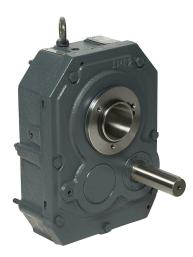
IronHorse heavy-duty shaft mounted gearbox, 9:1 ratio, 1-1/8in shaft input, tapered bore, maximum motor 10hp, 1-15/16in maximum output shaft diameter, size 2 frame, cast iron housing.
