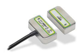
IDEM safety switch set, non-contact magnetic, rear mount, (2) N.C. safety output(s), (1) N.O. monitoring output(s), 316 stainless steel housing, 50 x 25mm, pigtail, 16.4ft/5m cable length.
