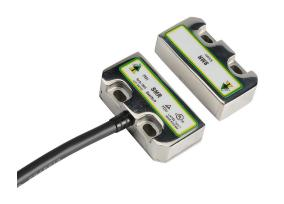
IDEM safety switch set, non-contact magnetic, (2) N.C. safety output(s), (1) N.O. monitoring output(s), 316 stainless steel housing, 50 x 25mm, 8-pin M12 quick-disconnect, 9.8in/250mm cable length.
