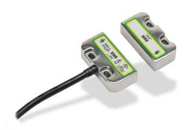
IDEM safety switch set, non-contact magnetic, (2) N.C. safety output(s), (1) N.O. monitoring output(s), 316 stainless steel housing, 50 x 25mm, pigtail, 32.8ft/10m cable length.
