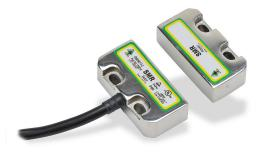
IDEM safety switch set, non-contact magnetic, (2) N.C. safety output(s), (1) N.O. monitoring output(s), 316 stainless steel housing, 50 x 25mm, pigtail, 16.4ft/5m cable length.
