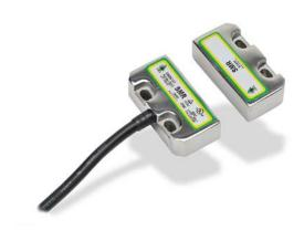
IDEM safety switch set, non-contact magnetic, (2) N.C. safety output(s), (1) N.O. monitoring output(s), 316 stainless steel housing, 50 x 25mm, pigtail, 6.5ft/2m cable length.
