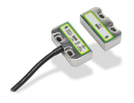
IDEM safety switch set, non-contact magnetic, (2) N.C. safety output(s), (1) N.O. monitoring output(s), 316 stainless steel housing, 50 x 25mm, pigtail, 6.5ft/2m cable length.
