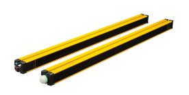
ReeR safety light curtain, sender/receiver pair, body protection, 24 VDC, 400mm resolution, 810mm protected height, 0-12m operating distance, safety category Type 4, configurable, IP65 IP67, (6) 5-pin and (1) 12-pin M12 quick-disconnect.
