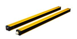
ReeR safety light curtain, sender/receiver pair, body protection, 24 VDC, 300mm resolution, 910mm protected height, 0-12m operating distance, safety category Type 4, IP65 IP67, (6) 5-pin and (1) 12-pin M12 quick-disconnect.
