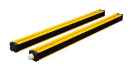
ReeR safety light curtain, active/passive pair, body protection, 24 VDC, 400mm resolution, 810mm protected height, 0-8m operating distance, safety category Type 4, IP65 IP67, (3) 5-pin and (1) 12-pin M12 quick-disconnect.
