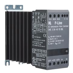
Eltwin SMC3-DOL series solid state contactor, 15A, (2) N.O. SCR switched, (1) Direct power poles, 400-480 VAC (50/60Hz) operating voltage, 24-60 VDC/24-480 VAC coil voltage.
