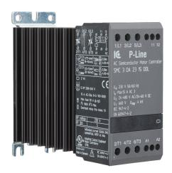
Eltwin SMC3-DOL series solid state contactor, 15A, (2) N.O. SCR switched, (1) Direct power poles, 208-240 VAC (50/60Hz) operating voltage, 24-60 VDC/24-480 VAC coil voltage.
