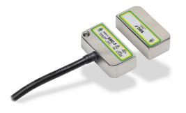
IDEM safety switch set, non-contact coded magnetic, rear mount, (2) N.C. safety output(s), (1) N.O. monitoring output(s), 316 stainless steel housing, 50 x 25mm, pigtail, 16.4ft/5m cable length.
