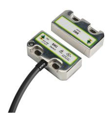
IDEM safety switch set, non-contact coded magnetic, (2) N.C. safety output(s), (1) N.O. monitoring output(s), 316 stainless steel housing, 50 x 25mm, 8-pin M12 quick-disconnect, 9.8in/250mm cable length.
