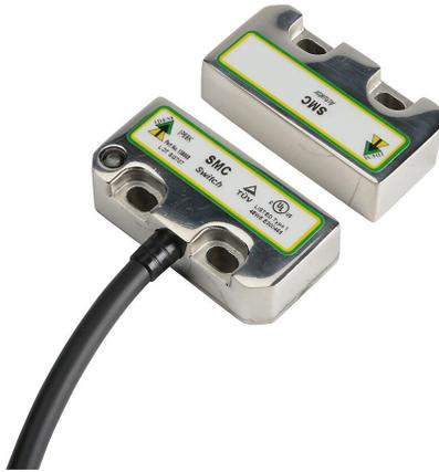
IDEM safety switch set, non-contact coded magnetic, (2) N.C. safety output(s), (1) N.O. monitoring output(s), 316 stainless steel housing, 50 x 25mm, 8-pin M12 quick-disconnect, 9.8in/250mm cable length.
