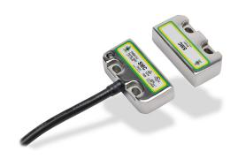
IDEM safety switch set, non-contact coded magnetic, (2) N.C. safety output(s), (1) N.O. monitoring output(s), 316 stainless steel housing, 50 x 25mm, pigtail, 32.8ft/10m cable length.
