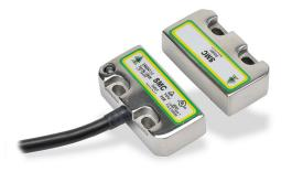
IDEM safety switch set, non-contact coded magnetic, (2) N.C. safety output(s), (1) N.O. monitoring output(s), 316 stainless steel housing, 50 x 25mm, pigtail, 16.4ft/5m cable length.
