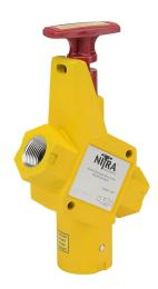
NITRA lockout valve, OSHA compliant, 1in female NPT inlet(s), 1in female NPT outlet(s), 1-1/4in female NPT exhaust(s), aluminum body.
