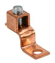
Penn-Union mechanical lug, offset tongue, copper-electrolytic, 70-90A, 1 openings, (1) 8 AWG solid-2 AWG stranded copper.
