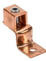
Penn-Union mechanical lug, offset tongue, copper-electrolytic, 225A, 1 openings, (1) 6 AWG-4/0 AWG stranded cooper.
