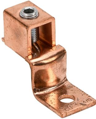
Penn-Union mechanical lug, offset tongue, copper-electrolytic, 225A, 1 openings, (1) 6 AWG-4/0 AWG stranded cooper.
