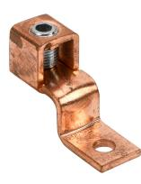
Penn-Union mechanical lug, offset tongue, copper-electrolytic, 125A, 1 openings, (1) 8 AWG solid-1/0 AWG stranded copper.
