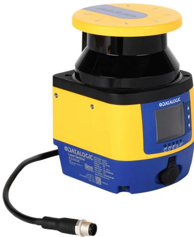
Datalogic safety laser scanner, area protection, 275 degrees operating angle, 0.05 - 3m operating distance, (1) safety zone, (2) warning zones, 24 VDC, safety category Type 3, IP65, (1) 4-pin and (1) 8-pin M12 quick-disconnect.
