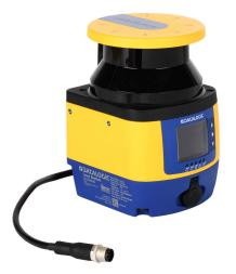
Datalogic safety laser scanner, area protection, 275 degrees operating angle, 0.05 - 3m operating distance, (1) safety zone, (2) warning zones, 24 VDC, safety category Type 3, IP65, (1) 4-pin and (1) 8-pin M12 quick-disconnect.
