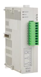
SOLO modular temperature controller, extension module, current, voltage, thermocouple or RTD input, (2) 3A SPST relays output, 24 VDC operating voltage, RS-485.
