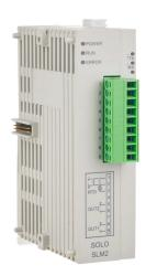
SOLO modular temperature controller, extension module, current, voltage, thermocouple or RTD input, 0-10 VDC, 0-10 VDC retransmission or 3A SPST relay output, 24 VDC operating voltage, RS-485.
