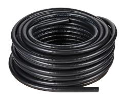
Electri-Flex Liquatite liquid-tight flexible metallic conduit, hot dipped galvanized steel, PVC jacket, copper braided shield, 1/2in trade size, black, UL-360 Listed, 100ft/30.4m coil length.
