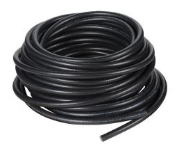
Electri-Flex Liquatite liquid-tight flexible metallic conduit, hot dipped galvanized steel, PVC jacket, copper braided shield, 3/8in trade size, black, UL-360 Listed, 100ft/30.4m coil length.
