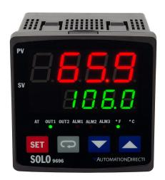
SOLO standard temperature controller, 1/4 DIN, 2-line LED, current, voltage, RTD, thermocouple or event input, (2) 11-15 VDC pulse, (2) 3A SPST relays output, 100-240 VAC operating voltage, RS-485.
