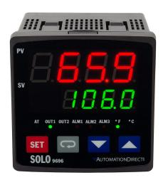
SOLO standard temperature controller, 1/4 DIN, 2-line LED, current, voltage, RTD, thermocouple or event input, (2) 5A SPDT relays, (2) 3A SPST relays output, 100-240 VAC operating voltage, RS-485.
