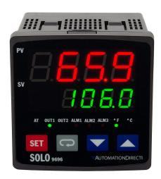
SOLO standard temperature controller, 1/4 DIN, 2-line LED, current, voltage, RTD, thermocouple or event input, (2) 5A SPDT relays, (2) 3A SPST relays output, 24 VDC operating voltage, RS-485.
